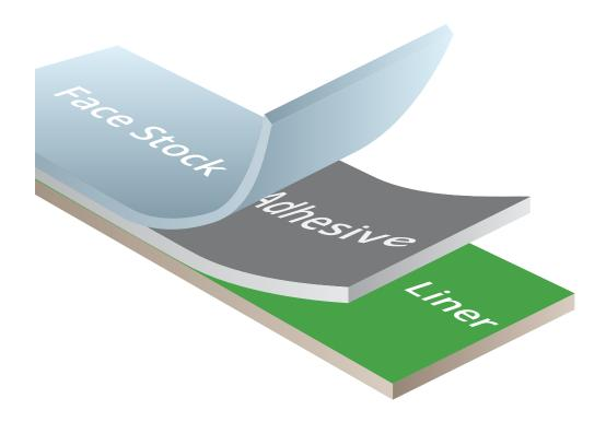
Face Stock: 5.0 mil polyimide masking tape offers excellent resistance to heat and chemicals. Specfically designed to protect the surface it is placed on. Ideal for marking gold contacts and other sensitive areas on printed circuit boards.
