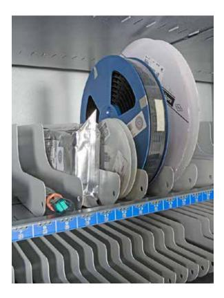
Positions with configurable separators
