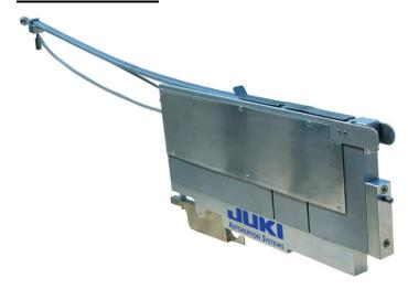
The "SIF" type feeders are designed for smaller ICs and advance parts using a small puff of air. The tube remains on the feeder until empty. An air fitting attaches to the back of the tube to blow the parts to the pick position.
