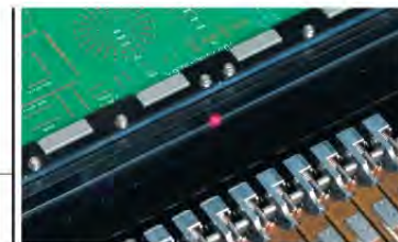
Feeder Position Indicator
