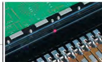
Feeder Position Indicator
